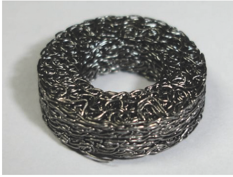
FIGURE 1: Pseudoelastic compressed SMA mesh washer isolator [21].
