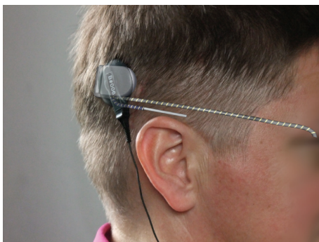
FIGURE 3: Illustration of the subdermal placement of the receiver coil and the power supply cable (white/grey) in relation to the epidermal transmitter coil (black) and cable leading to the power supply in the patient's pocket.
