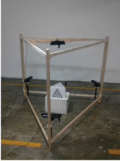
FIGURE 8: Experimental environment, image data acquisition system used in this study. The object is a triangular prism calibration body (1) designed with a designed calibration board. (2) and (3) are Kinect equipment to obtain the images. Four Kinects as shown in Figure 8 obtain images in four different views by facing a surface of triangular prism.
