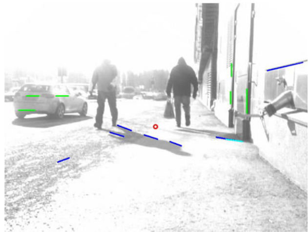
Fig. 3 An image from the validation process showing how a false vanishing point location ( red dot ) was obtained
