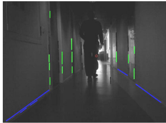
Fig. 5 Calculation of the central vanishing point (red dot) is largely tolerant to dynamic objects in the scene
