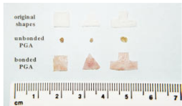
Figure 9. Photograph demonstrating final gross shapes of tissue constructs engineered on either unbonded PGA matrices or bonded PGA matrices (bonding PLLA mass = 136% of the initial PGA mass) fabricated into specific geometries. Tissues were allowed to develop for 8 weeks in vitro .
