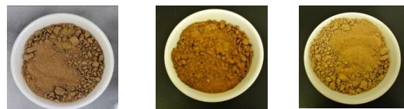
Figure 14. Soil tests(left: naturally dry; middle: mixed with deionized water; right: absolutely dry)
