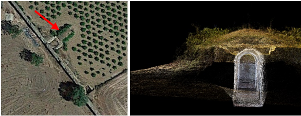
Figure 2. Area of Roman Dam captured with TLS (left), red arrow indicating location of subterranean structure; front view, point cloud render of subterranean structure (right)
