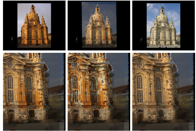
Figure 8: Lighting changes in the Church data set. Top row: transition at 0%, 50%, and 100% transition time. Bottom row: close-up at 50% with soft z-buffer and alpha normalization (left), without soft z-buffer (middle), and without alpha normalization (right).
