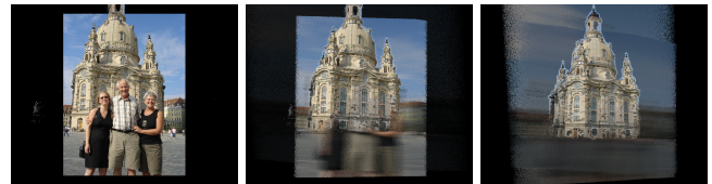
Figure 7: Beginning of a transition in the Church data set. The figure shows the original starting image (left) and renderings at 30% and 50% of the transition. Note how the occluding persons dissolve in the ambient point cloud. Holes in the church façade are filled using alpha normalization.
