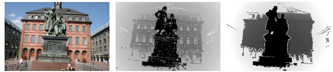
Figure 3: One of the input images in the town square data set and the corresponding raw (middle) and final depth map including the background plane (right).
