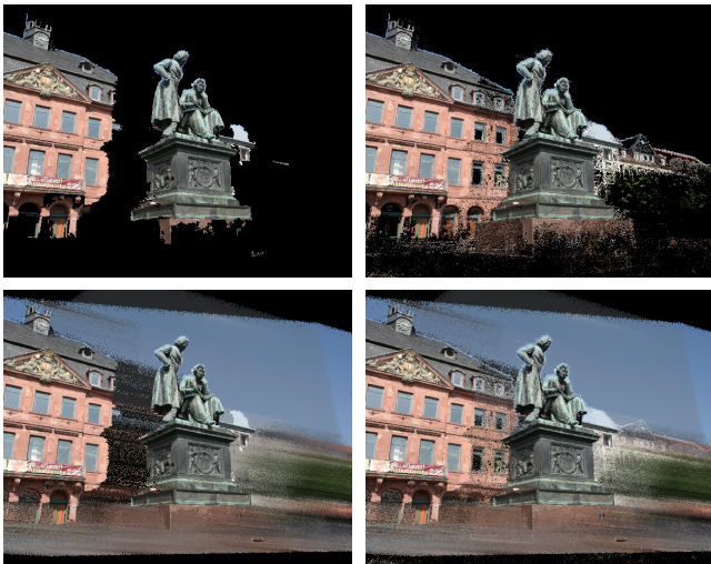
Figure 6: Town Square data set using just certain geometry (top-left), geometry with global point cloud (top-right), geometry with ambient point cloud (bottom-left), and all combined (bottom-right).
