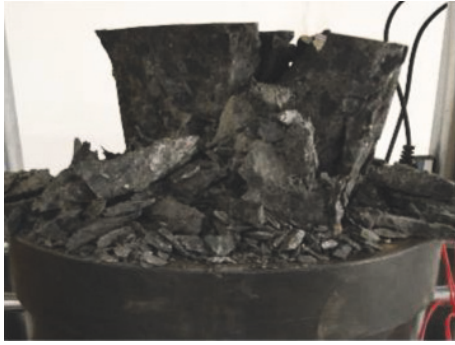
FIGURE 3: Failure mode of C100 UHSC.
