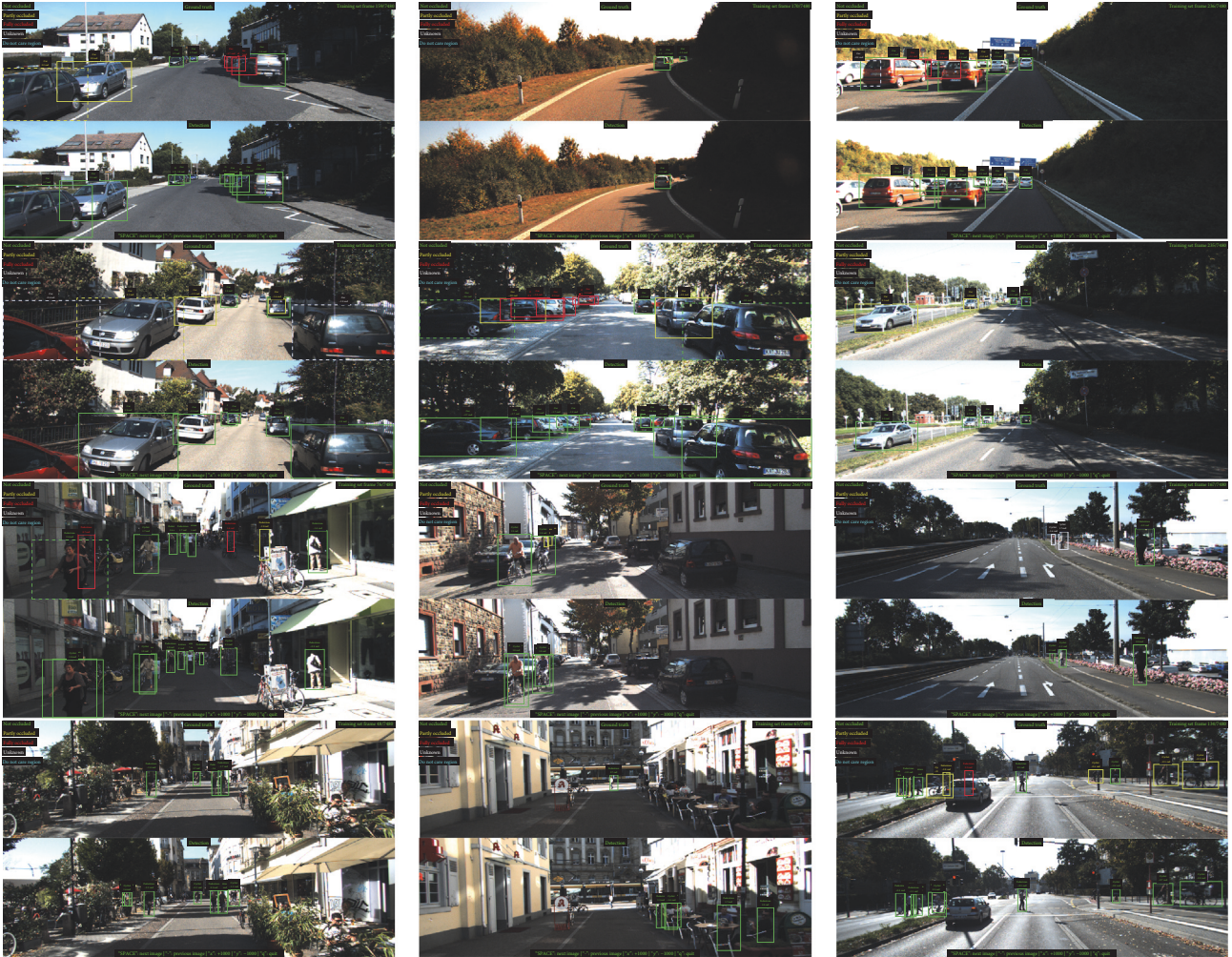
FIGURE 7: The visual results of our object detection framework. The odd rows are the ground truth bounding box while the even rows are detection bounding box. Different colors indicate different difficulties. Green means not occluded, yellow means partly occluded, and red means fully occluded. The first four rows are the results of Cars, while the second four rows are the results of Pedestrian and Cyclist.
