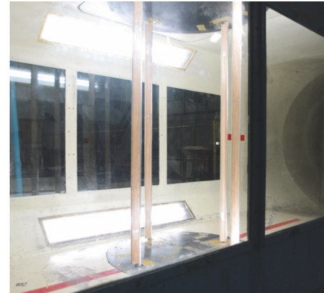
(a) Iced 4-bundled conductors
