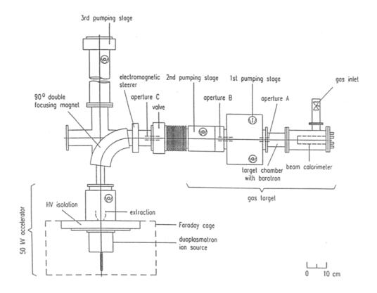
Fig. 1.— Schematic diagram of the 50 KV LUNA facility.
