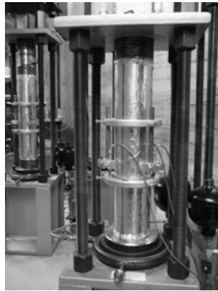
Figure 3. Compressive creep devices with sealed cylindrical samples
