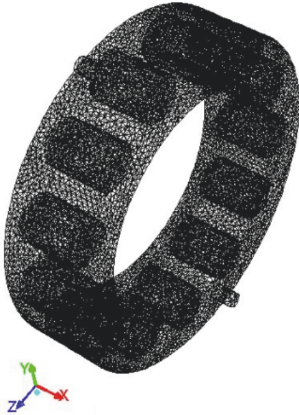
FIGURE 3: Meshing model of bearing cavity.
