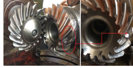
FIGURE 3: Tooth surface pitting.
