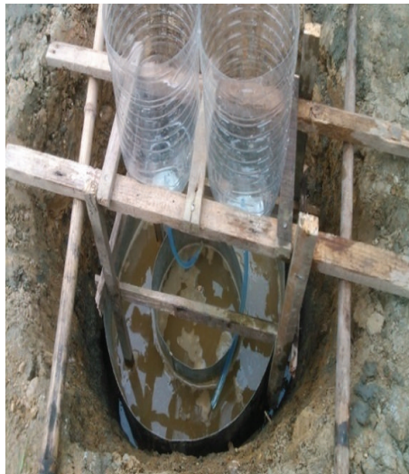
FIGURE 6: Simple apparatus of double-ring infiltrometer.
