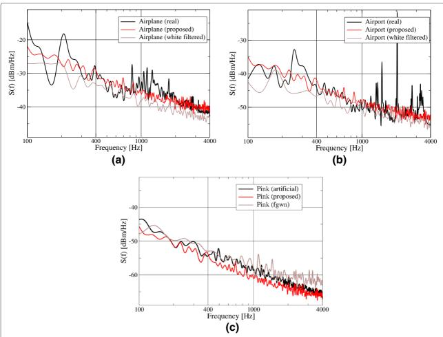
Figure 2 PSD obtained from the real, the proposed and fgwn methods 1/f noise samples. (a) Airplane (fgwn), (b) Airport (fgwn), (c) artificial pink.
