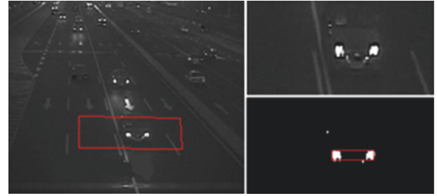
FIGURE 8: Frame 567: left, inverse projection plane set; right top, building the inverse projection map; right bottom, rough matching.
