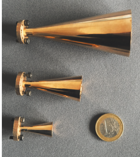
FIGURE 3: 3D printed horns antennas, from top E-, D-, and H-band.
