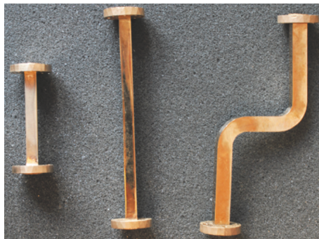
FIGURE 4: 3D printed waveguides, from left: 50 mm straight waveguide, 100 mm straight waveguide, and bend waveguide.
