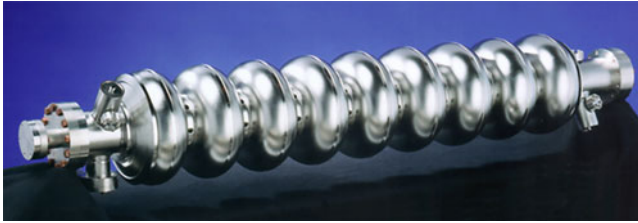
Figure 4. Picture of a TESLA-type 9-cell superconducting niobium cavity. The length is 1 m. Courtesy: DESY.
