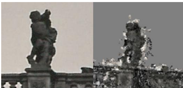
Figure 4. Comparison of a segment originated from a historical image (left) and a point cloud (right)
