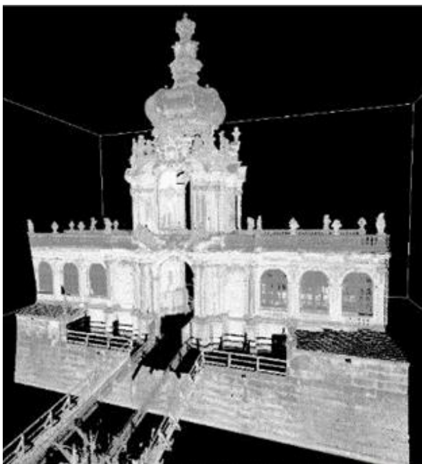
Figure 12. Point cloud based on terrestrial laser scanner data
