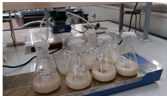
Fig. 1 Biodegradation of diazinon using wet cells of S. cerevisiae at different pH, concentration and reaction times
