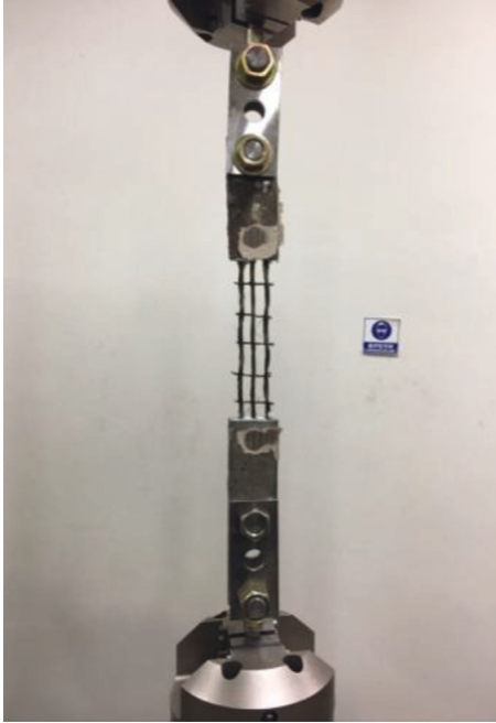
FIGURE 2: Direct tensile test of FRP fabric.
