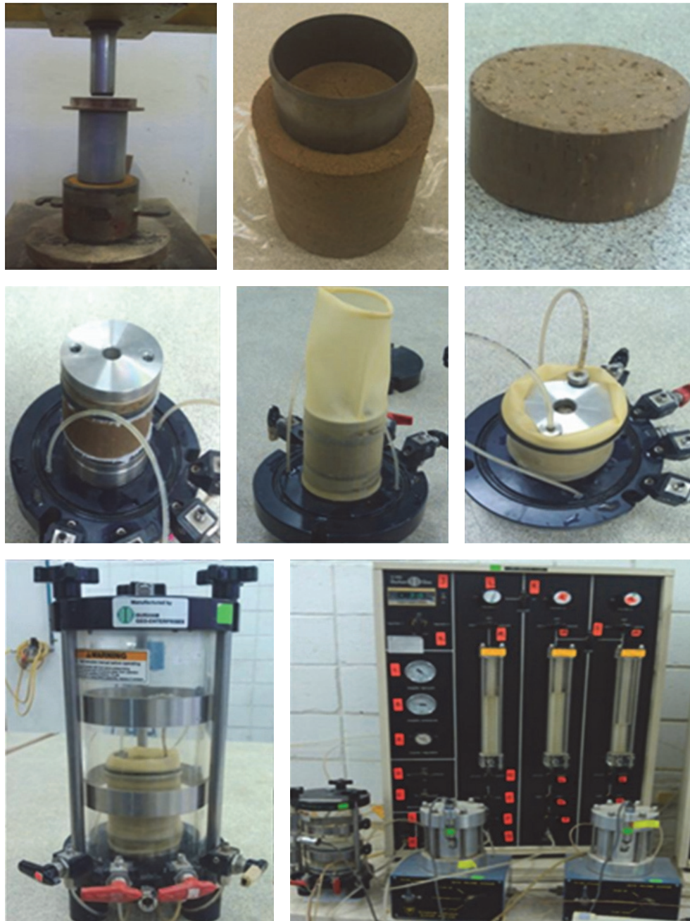
FIGURE 5: Sample preparation procedures for hydraulic conductivity test in flexible membrane apparatus.
