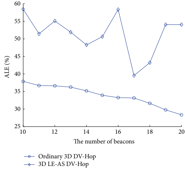
FIGURE 12: ALE on locations based upon the number of beacons in 3D environment.
