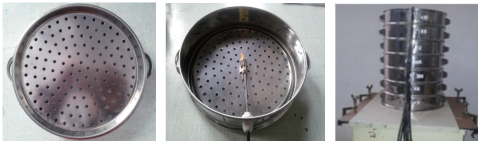
FIGURE 9: Thin layer drying experiment boxes and sensor installation position.
