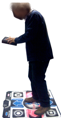
Figure 9:1 - Photograph of the prototype system in use. As can be seen from the photograph, the dance mat has nine squares and two buttons located at the top of the dance mat.
