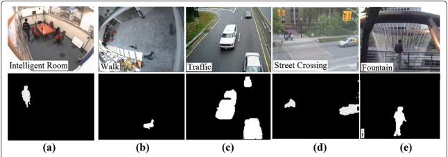
Figure 7 Detection results of proposed algorithm. (a,b) Two indoor sequences with shadows. (c) A sequence with varying illumination. (d,e) Two environments containing repeated motions in the background.
