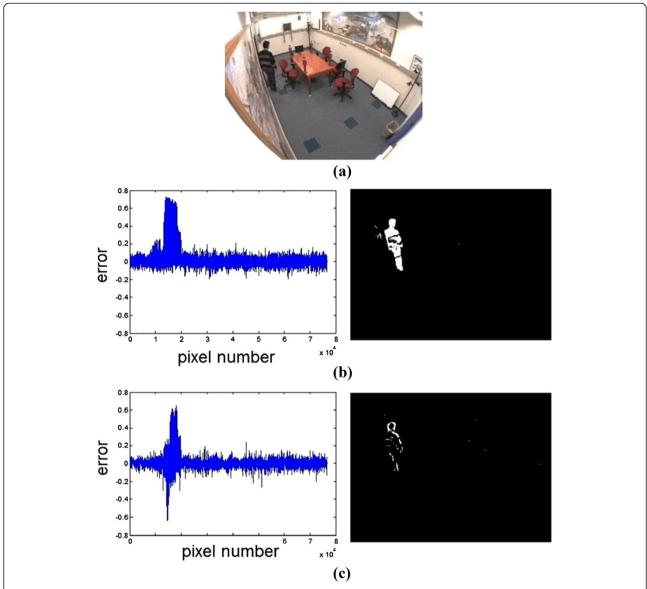
**Figure 4 ANC-based motion detection. (a)** One frame of an indoor video sequence. **(b)** The output of algorithm using one background frame and a frame including moving object. **(c)** Output of ANC algorithm using two consecutive frames both containing moving objects.
