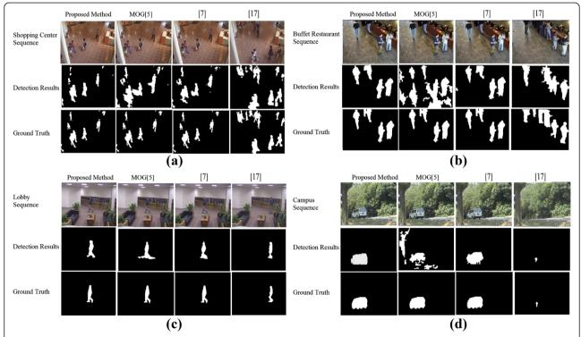
Figure 6 Detection results of proposed algorithm compared with three earlier works introduced in [5,7,17]. (a,b) Two indoor sequences with shadows and bootstrapping. (c) An office building with switching on/off light. (d) An environment containing repeated motions in the background due to waving trees.
