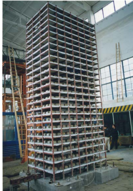
Fig. 15 The composite model structure: (a) SF and CT fixed on the base (concrete slabs yet cast); and (b) the completed model structure installed on the shaking table with additional mass
