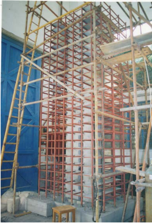
Fig. 15 The composite model structure: (a) SF and CT fixed on the base (concrete slabs yet cast); and (b) the completed model structure installed on the shaking table with additional mass
