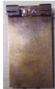
Fig. 4 Photograph of prototype of the proposed balanced antenna design.
