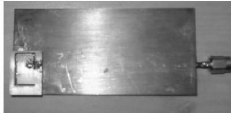
Fig. 3. The prototype (loaded) antenna structure.
