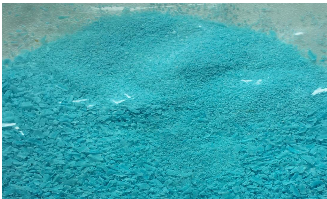
[Fig. 5.31 Batch -11 showing uniform colour dispersal of Methylene blue over the MCC through twin screw extrusion using standard mixing configuration]
