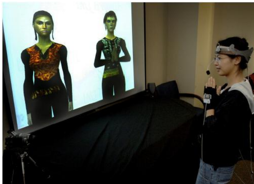
Figure 15. The immersive virtual reality social conversational protocol training system. This system uses two networked PCs for speech and gesture recognition, and visual rendering. A data projector displays the life-sized virtual
