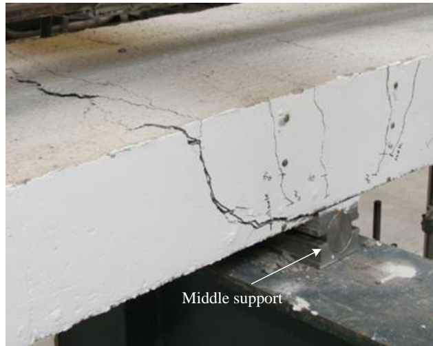
Figure 3-13: Flexure-shear failure at middle support of slab C-B-UU
