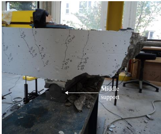
(a) Flexural-shear failure at middle support of slab C-C-OO
