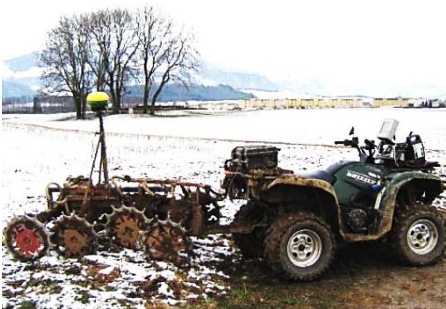
Figure 3.5 The ARP© system towed behind a quad bike (Dabas and Gruel 2009).
