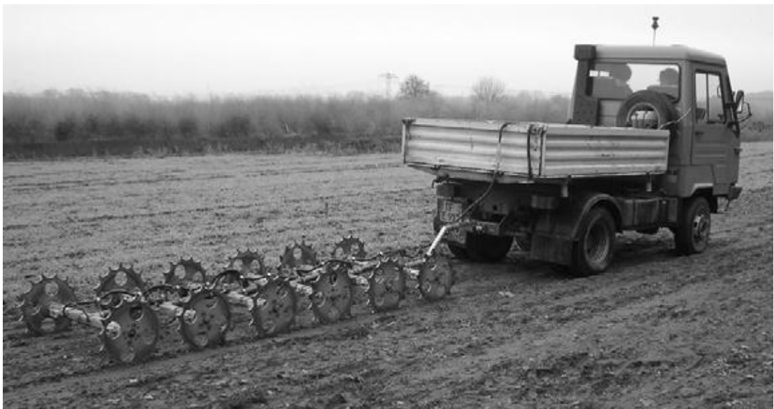
Figure 3.8 The Geophilus Electricus being towed behind a small lorry and its position recorded by a total station (prism mounted on top of the cab) (Simpson et al. 2010 2200).
