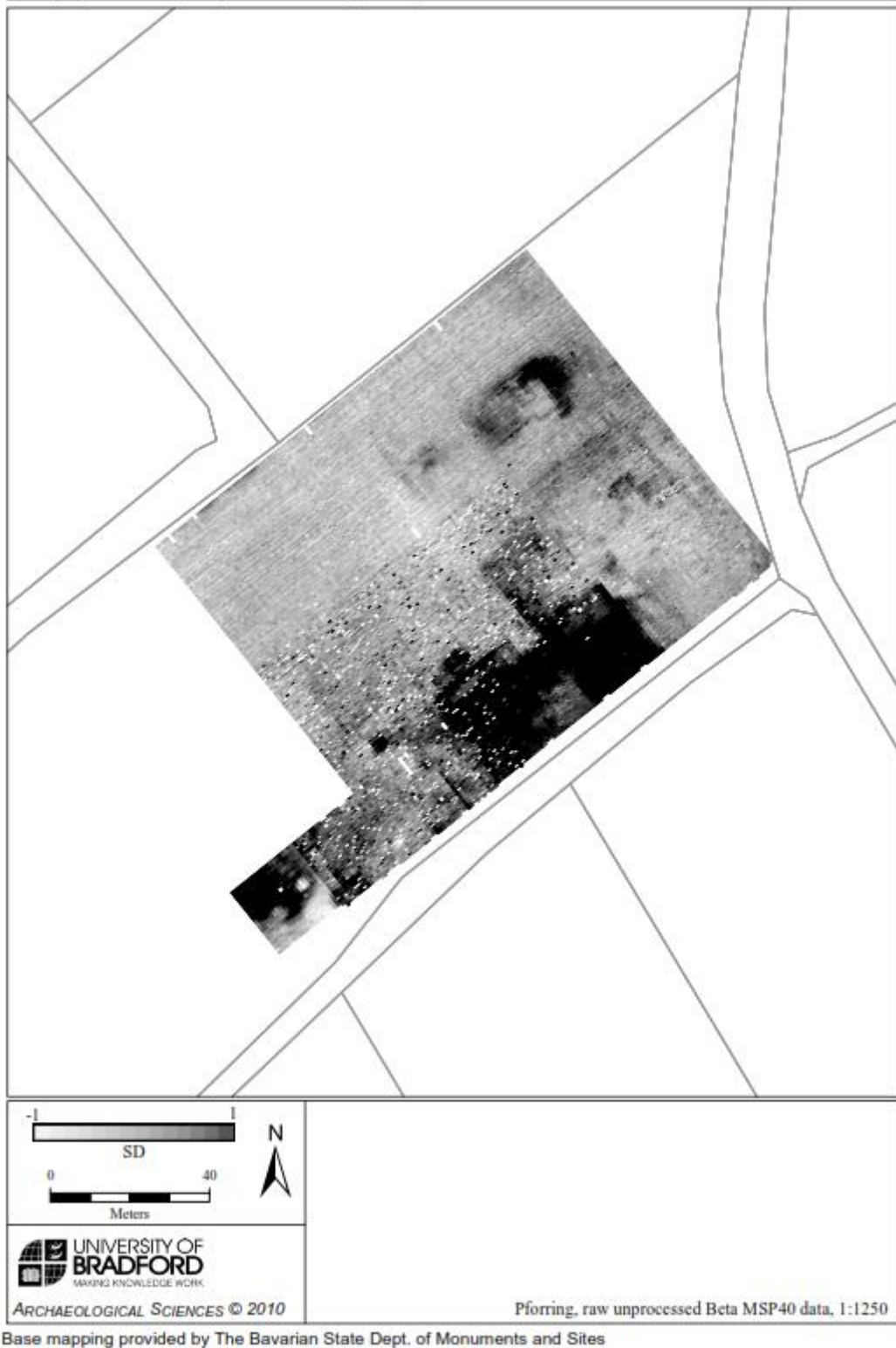
Figure 5.41 Processed earth resistance data (Beta) from Pförring Area C.
