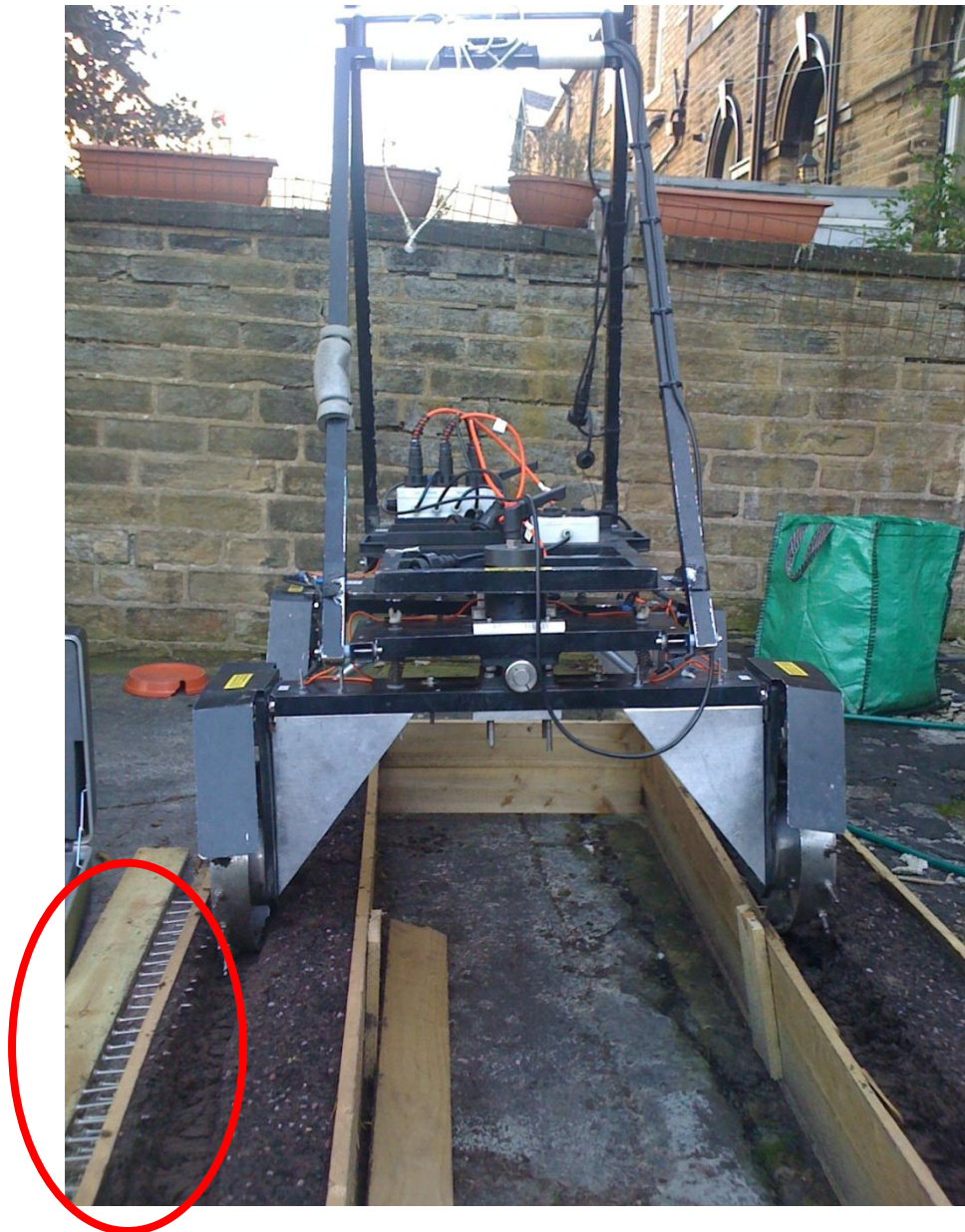
Figure 4.55 A photograph of the MSP40 as it was pulled past the banks of electrodes (highlighted in red).
