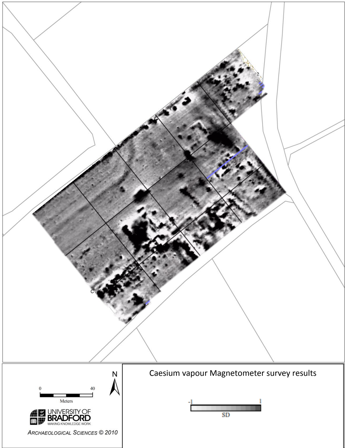
Figure 5.45 Processed caesium vapour magnetometer survey from Eining Area B. Data provided by The Bavarian State Department of Monuments and Site.
