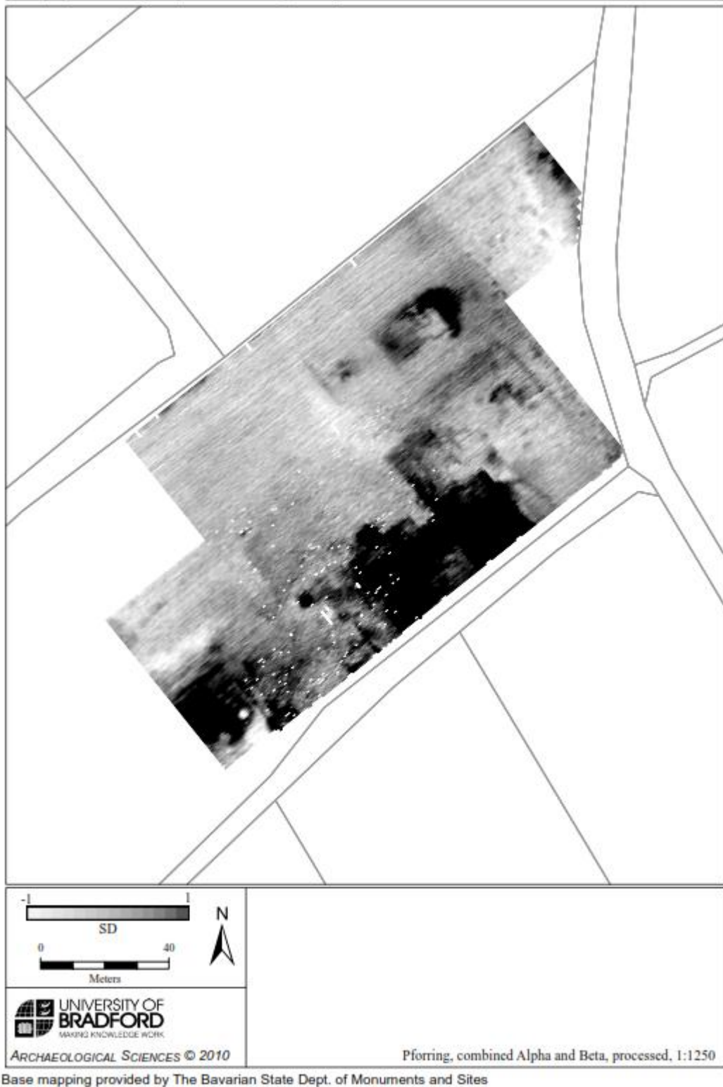
Figure 5.43 Processed earth resistance data (combined Alpha and Beta data sets) from Pförring Area C.
