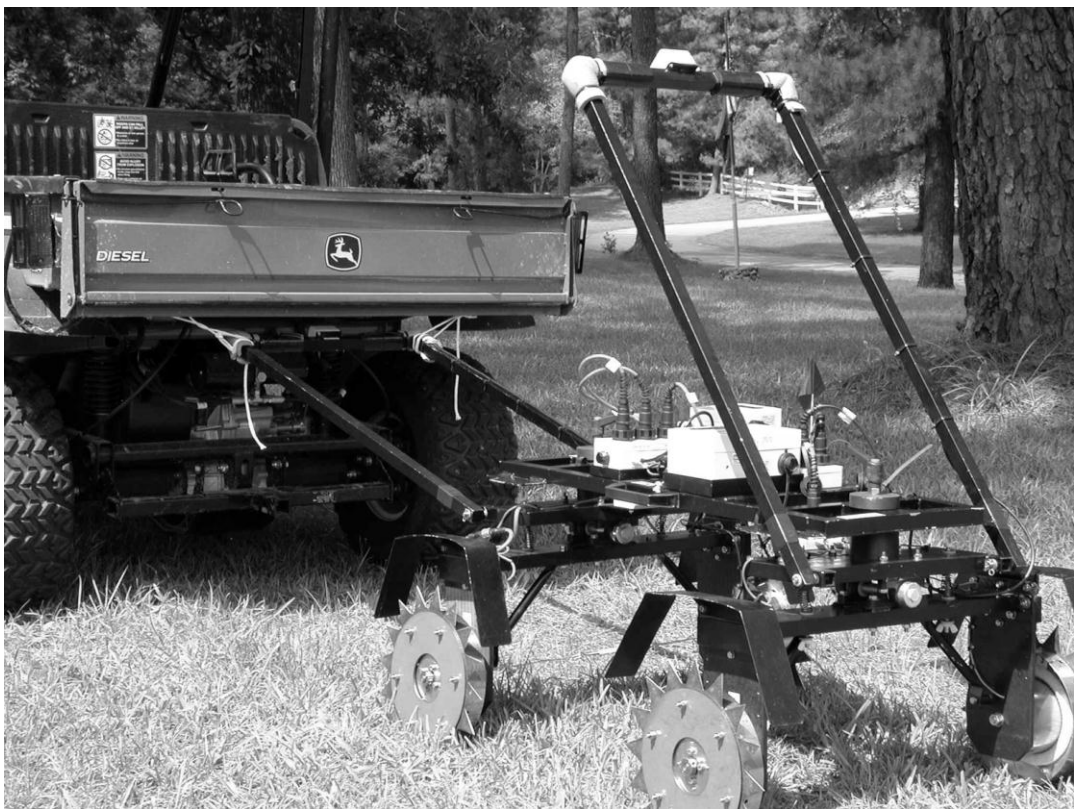
Figure 3.30 The MSP40 with a toothed wheel configuration being towed behind a vehicle (Somers 2010).
