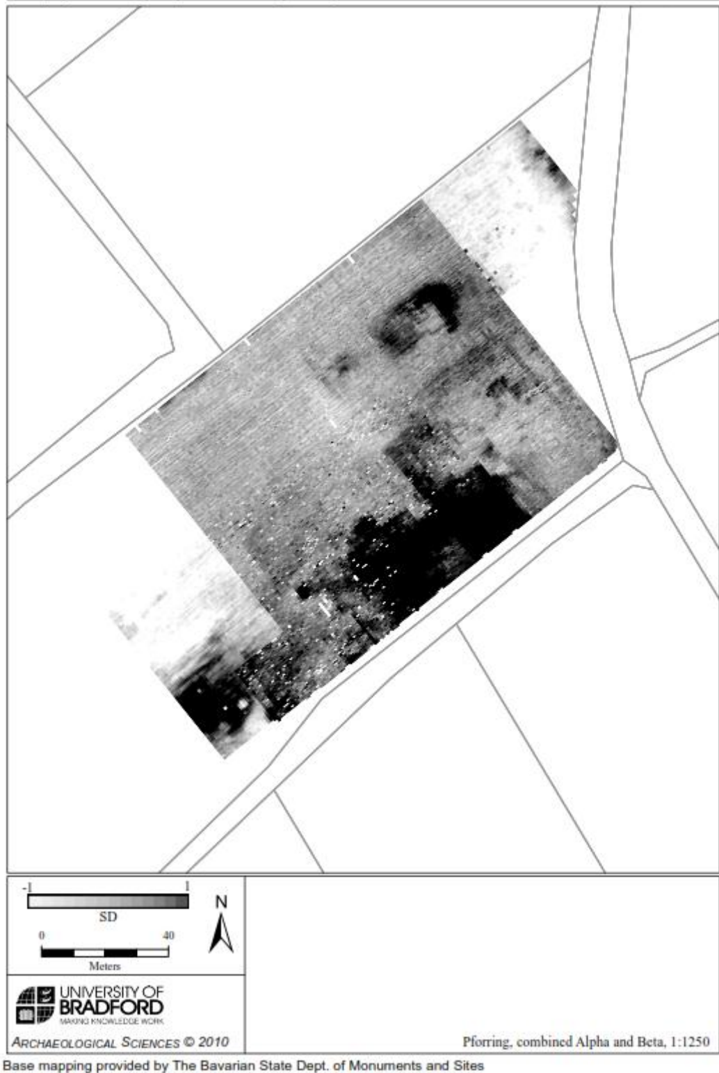
Figure 5.42 Minimally processed earth resistance data (combined Alpha and Beta data sets) from Pförring Area C.
