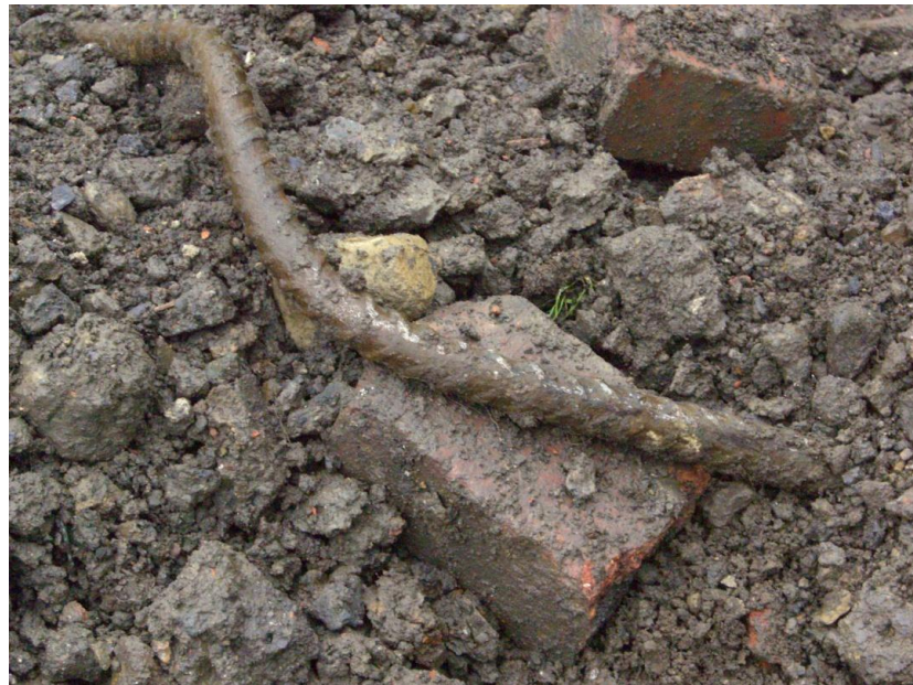
Figure 3.52 Brick and steel rebar that have strong localised magnetic fields.
