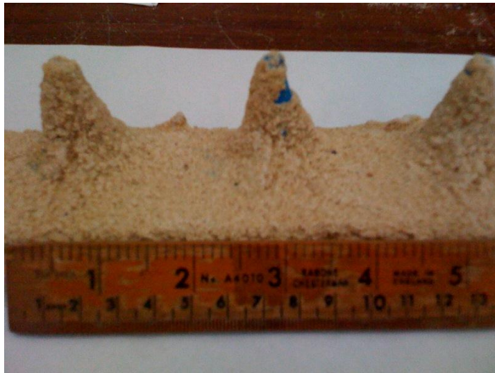
Figure 4.38 A photograph of the stone casts of the normal spiked wheel experiments with the crushed blue chalk adhering to the cast.
