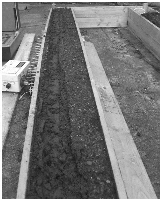
Figure 4.57 A photograph of the rut left by the MSP40 running alongside the electrode bank.
