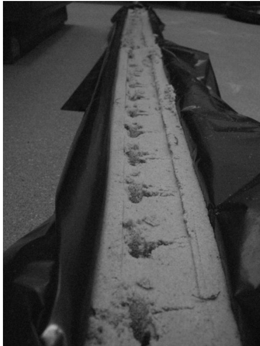
Figure 4.36 The impressions left in the sand from the normal spiked wheel, the spikes cut and ripped the sand surface whilst the wheels compacted the sand.
