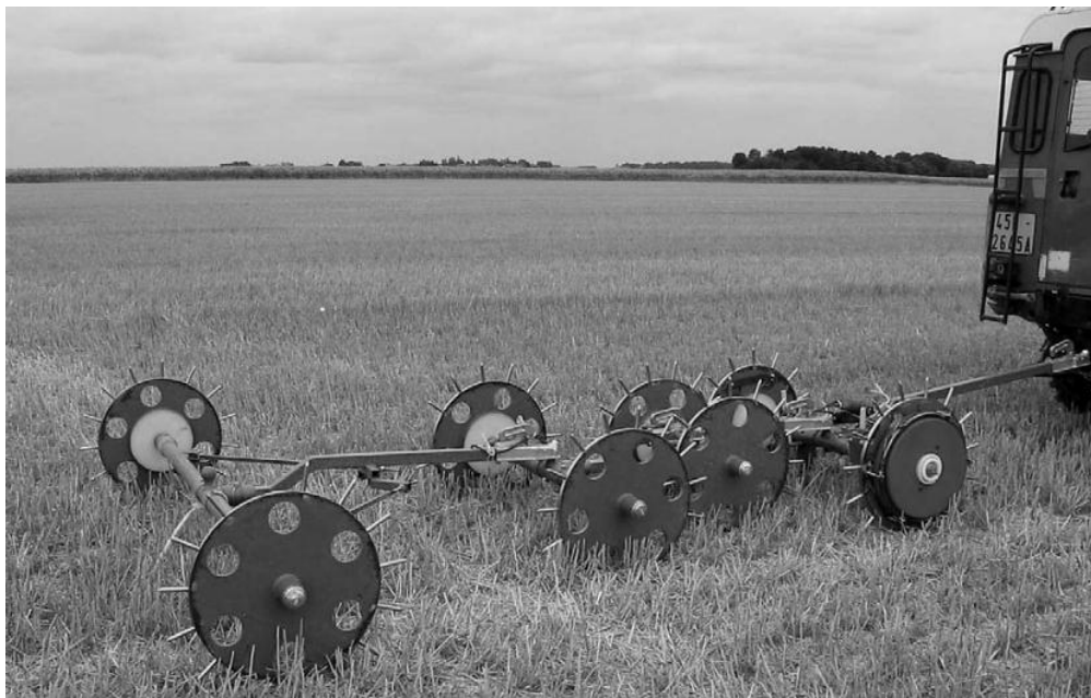
Figure 3.2 The MUCEP array towed behind a Land Rover (Samouëlian et al. 2005).
