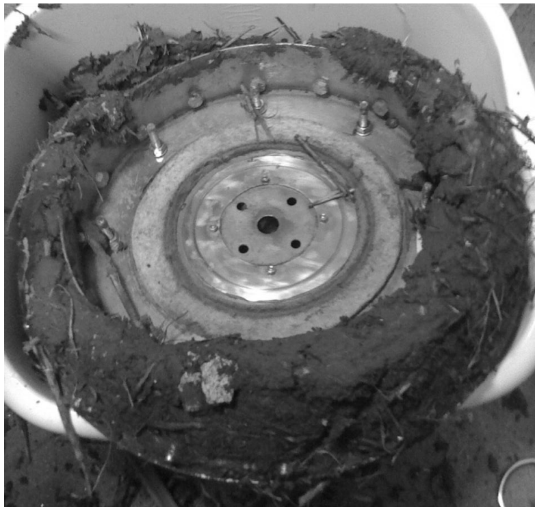
Figure A.4 A mud encased wheel from the MSP40 after a field trial at Towthorpe 18 round barrow.
