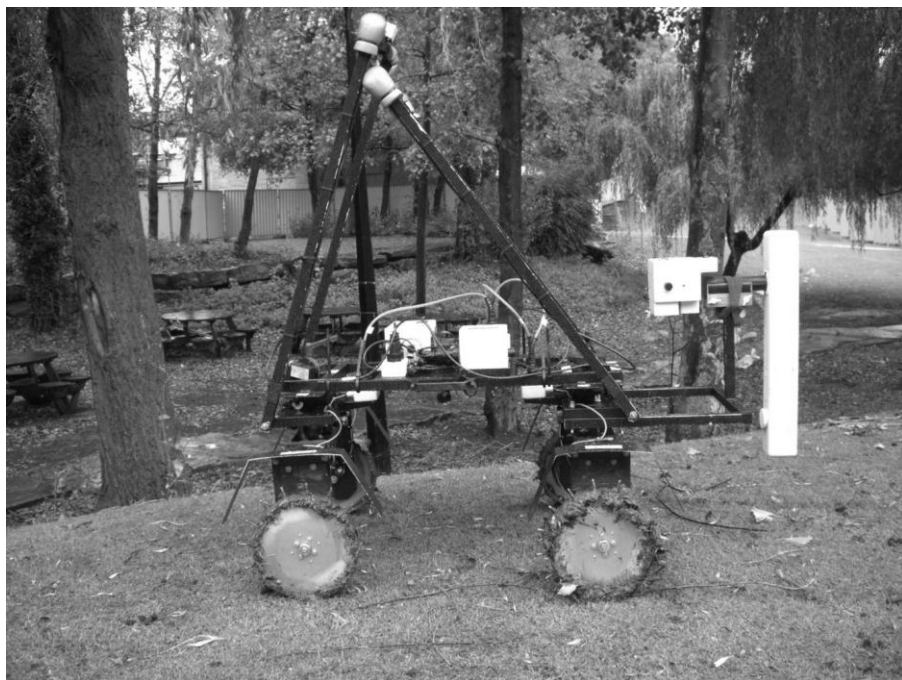
Figure 4.45 The normal spiked wheel rims 'caked' with material after partially surveying a 20m grid.
