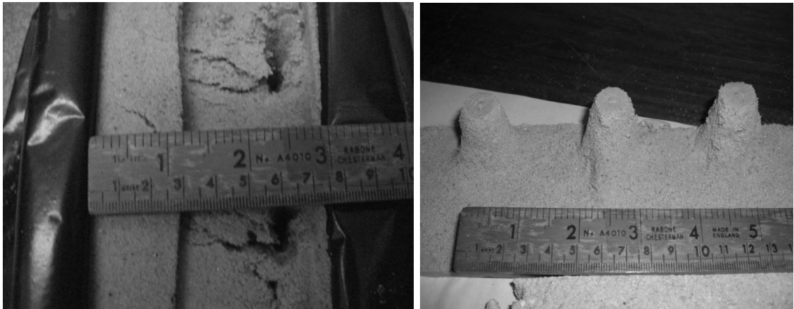
Figure 4.37 A close up of the surface 'tearing' and the results of the unsuccessful silicon resin experiment.
