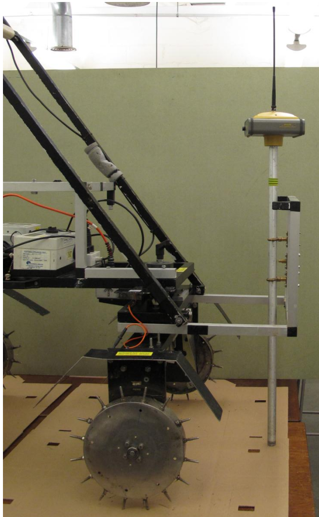
Figure 3.19 The 1 st generation rear mounted GPS unit attached to the detail pole on the MSP40 (Sparrow 2013).
