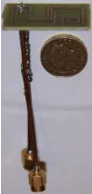
Figure 1b. RFID tag antenna for metal surface: antenna prototype with Alien chip (Higgs-2).
