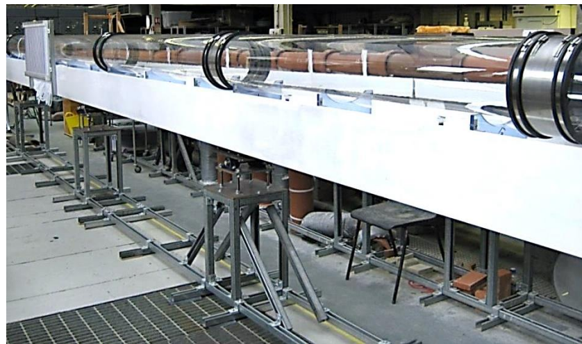
Figure 3.3 Arrangement of 290mm diameter perspex pipe.
