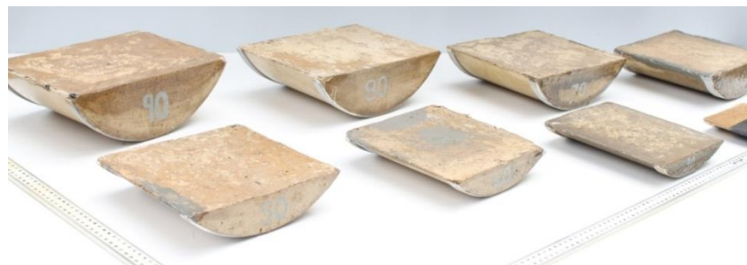
Figure 3.7 Model blockage samples for 290mm diameter pipe.
