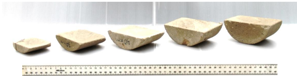
Figure 3.6 Model blockage samples for 150mm diameter pipe.
