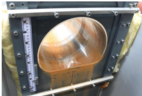
Figure 3.5 End gate of 290mm diameter perspex pipe which was used for uniform water depth control.
