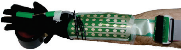
Figure 1: Electrode array with data glove and electrogoniometer used for stimulating and tracking hand and wrist movement.
