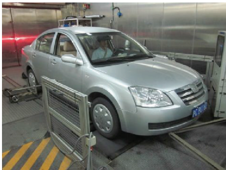
FIGURE 13: Photo of real car chassis dynamometer test.
