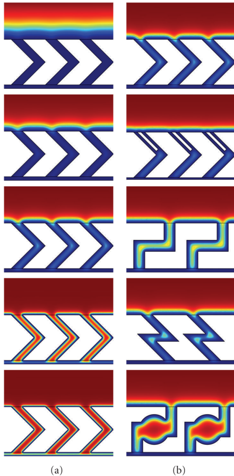
FIGURE 6: Simulation of the electron density by sheath model penetration of plasma into slots (a) at various plasma densities, and impact of the slot geometry (b) on plasma presence in the slot. The plots from top to bottom in column (a) represent simulation results at various bulk plasma density, that is, 1 \times 10^9 \text{ cm}^{-3} , 5 \times 10^9 \text{ cm}^{-3} , 1 \times 10^{10} \text{ cm}^{-3} , 5 \times 10^{10} \text{ cm}^{-3} , and 1 \times 10^{11} \text{ cm}^{-3} . Plots in column (b) are computed at bulk plasma density 1 \times 10^{10} \text{ cm}^{-3} .
