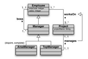
*Example 5.* Consider the UML class diagram in the picture above representing (part of) a company information system. According to the diagram, all managers are employees and are partitioned into area managers and top managers. In OWL 2 QL, we can write
