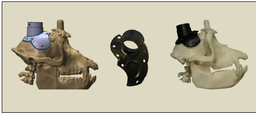
Fig. 4. Pictures showing the building up of another chronic recording chamber to access a different area (thalamus) after completing the investigations in the premotor cortex (see text). On the left, the picture shows a simulation of the new chronic recording chamber before it was fabricated. On the right the picture shows the real chamber in tekapeek and placed on the 3D replicate printing of the monkey's skull (Mk-LI).
