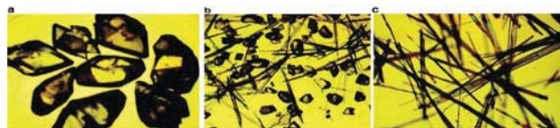
Fig. 2 (a) Morphology of form A of 3-acetyl coumarin. (b) Morphology of the form A and B at 5 °C depicting concomitant polymorphism. (c) Morphology of form B at 23 °C. Reprinted with permission from. 32 Copyright ©2004 American Chemical Society.
