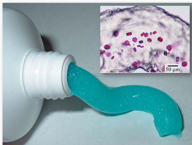
Figure 6 The cubic phase is viscous and sticky; it has the consistency of thick toothpaste. The particular toothpaste used in this figure contains small white crystals. This is exactly what is sought when in meso crystallization trials are set up. The inset shows crystals of the integral membrane light-driven proton pump bacteriorhodopsin growing in the lipid cubic phase. The analogy between the toothpaste and the crystal-laden mesophase is obvious.
