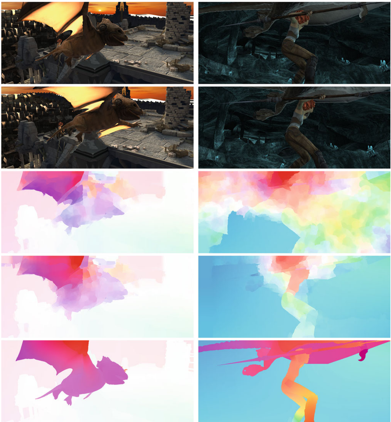
Fig. 10 Example results on MPI Sintel dataset. From top to bottom : first frame, second frame, results by Classic+NL (5-level), results by Classic+NLP (7-level), and ground truth. The asymmetric pyramid leads to a significant improvements in large regions undergoing large motion (head of the dragon on the left and background on the right ).
