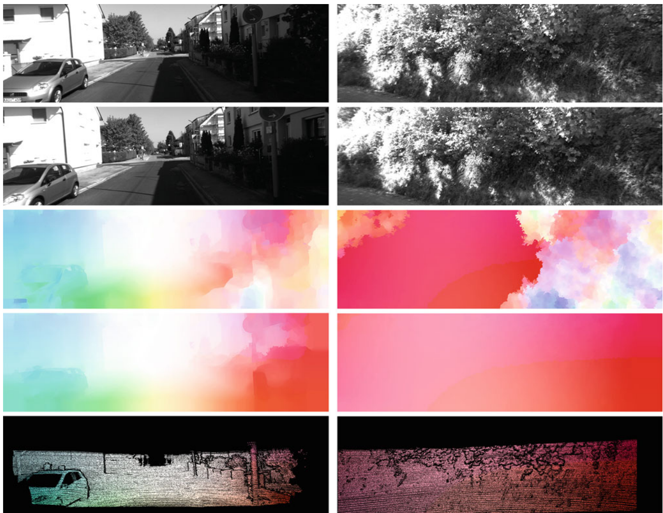
Fig. 11 Example results on the KITTI dataset. From top to bottom : first frame, second frame, results by Classic+NL-fast (5-level), results by Classic+NL-FastP (7-level), and ground truth for the non-occluded feature points. EPE results in non-occluded sparse feature points: “000002”
