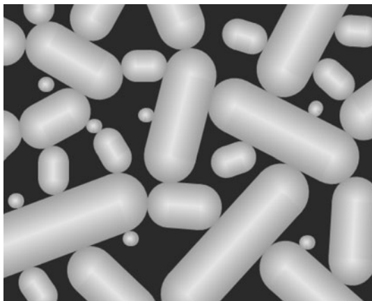
Fig. 2 A schematic picture of random porous structure (pore wall roughness is not shown)
