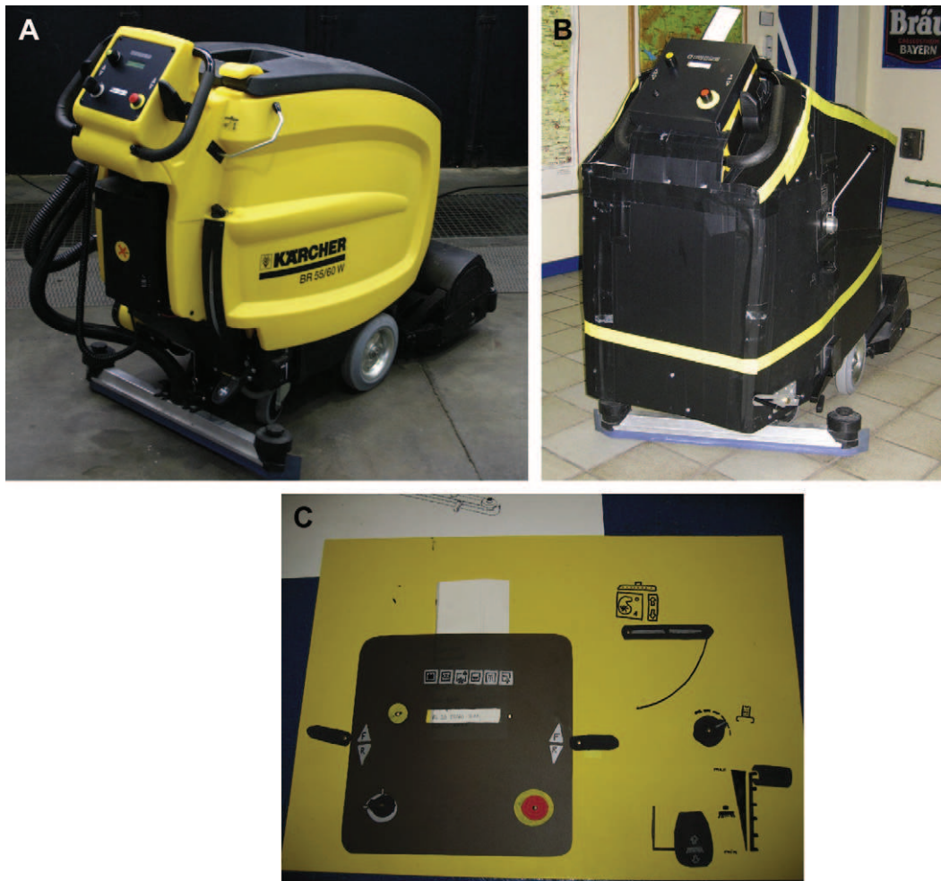
Fig. 2. Prototypes of floor scrubber: (a) high-fidelity, (b) medium-fidelity, and (c) low-fidelity.
