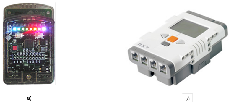
Figure 6.6: Devices used for the activity recognition: a) sunSPOT, b) Lego Minstorm NTX
