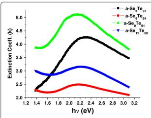
**Figure 6** Variation of extinction coefficient (k) with incident photon energy (hv) in a-Se $_x$ Te $_{100-x}$  thin films composed of aligned nanorods.
