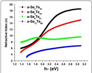
**Figure 7** Variation of refractive index (n) with incident photon energy (hv) in a-Se<sub>x</sub>Te<sub>100-x</sub> thin films composed of aligned nanorods.
