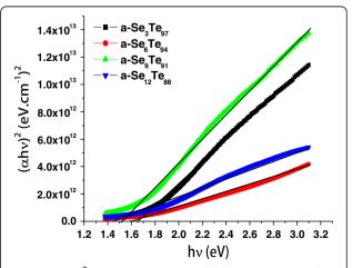
Figure 5  $(ahv)^2$  against photon energy (hv) in a-Se<sub>x</sub>Te<sub>100-x</sub> thin films composed of aligned nanorods.
