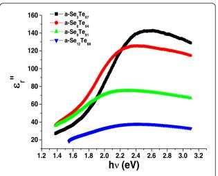
Figure 9 Variation of dielectric constant imaginary part with incident photon energy in a-Se $_x$ Te $_{100-x}$  aligned nanorod thin films.  $\in$ ,", imaginary part of the dielectric constant; hv, incident photon energy.
