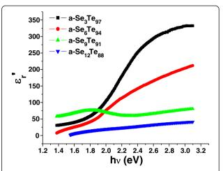
Figure 8 Variation of dielectric constant real part with incident photon energy in a-Se<sub>x</sub>Te<sub>100-x</sub> aligned nanorod thin films.  $\epsilon_r'$ , real part of the dielectric constant; hv, incident photon energy.
