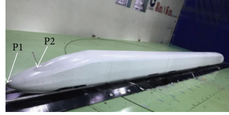
FIGURE 6: The 1:8 scale train model in the aerodynamic force wind tunnel.
