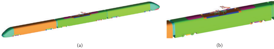
FIGURE 34: The train model after optimization for aerodynamic noise performance: (a) entire vehicle and (b) magnified view.
