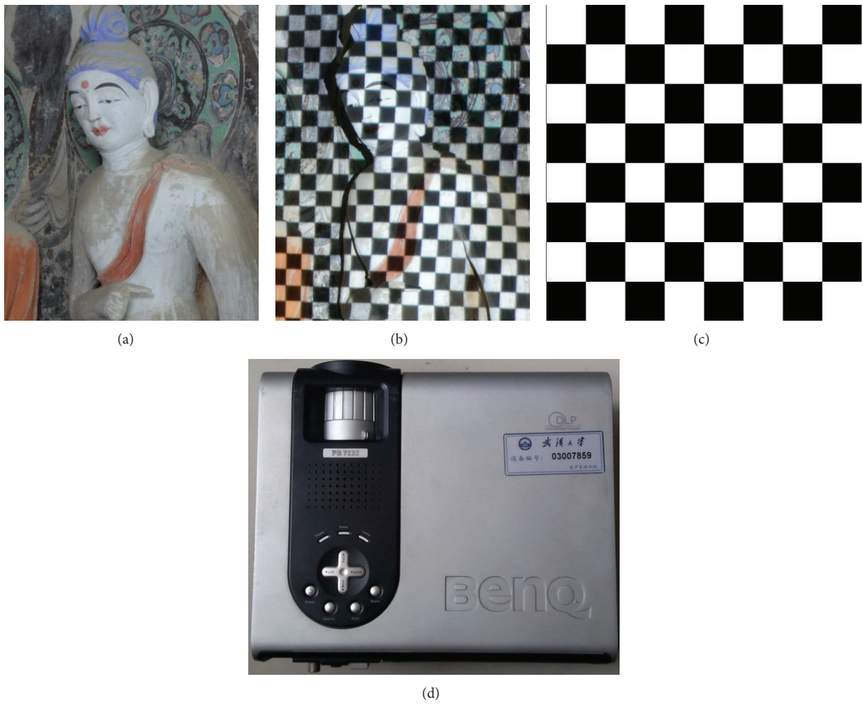
FIGURE 3: Intensive feature point generation method: (a) poor texture, (b) square projection, (c) the checkerboard, and (d) the projector.
